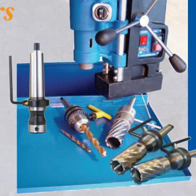
Need to use *twist drills* with your d2 drill? Need to use annular cutters with your CNC or Bridgeport? With our optional industrial arbors and 2MT-1/2"Drill Chuck now you can! SteelMax industrial arbors let you easily adapt our premium m2AL cutters to a variety of machinery, including CNC, lathe's, stationary drill presses and similar equipment. With our integrated coolant collar, cutter performance and cutter life is assured!
