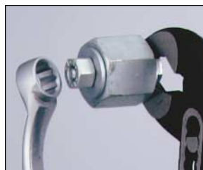
Washer Dishing/Belling Demonstration
