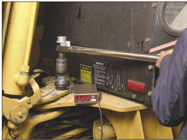
On-Site Torque Test
