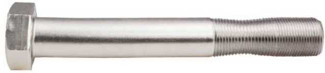
Permanently stretched capscrew
