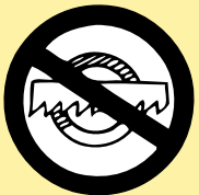
Teeth too small, no chip clearance, teeth clog
