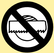
Teeth too coarse, straddle work, strip teeth
