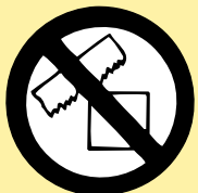
Angle of cut too abrupt, liable to strip teeth
